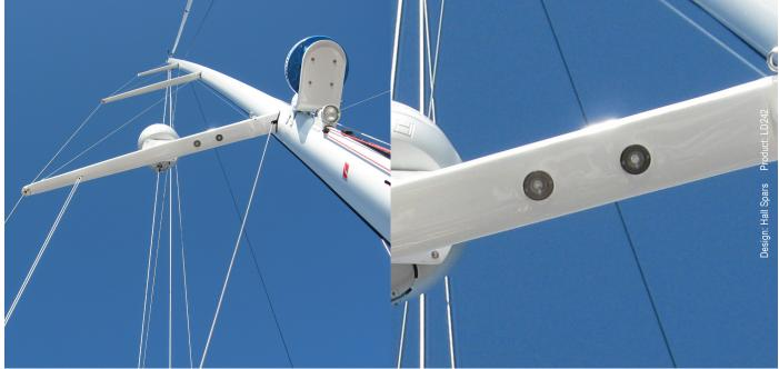
This has been specifically designed for use on yacht spreaders to illuminate the deck or other spreaders below. It is fitted with the latest LED technology and machined from a solid billet of high grade aluminium. This is hard anodised making it resistant to harsh sea environments. The narrow 12 degree beam will light a deck from 9m.
